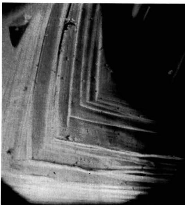
Fig. 10. Growth layers on the (111) face \times (395).
